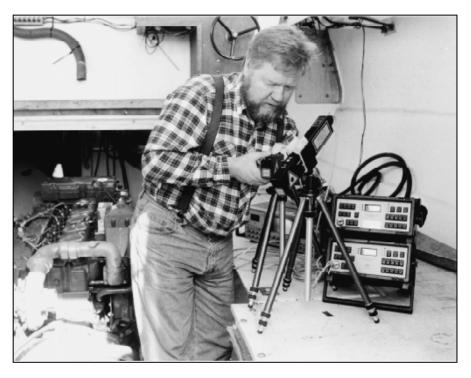
Two Torsional Vibration Meters Type 2523 being prepared for a marine application. The operating principle ensures that the instrument can be employed even in severe environments with maintained confidence in the results
